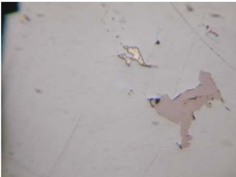
e) Native gold and pyrrhotite in arsenopyrite. Costești ores. N II, 190x magnification, oil immersion.
