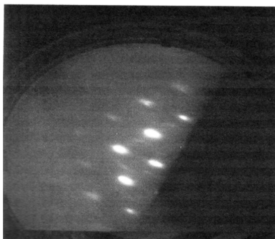
Fig. 1. Representation of an InAs/GaAs (001) Rheed pattern.
