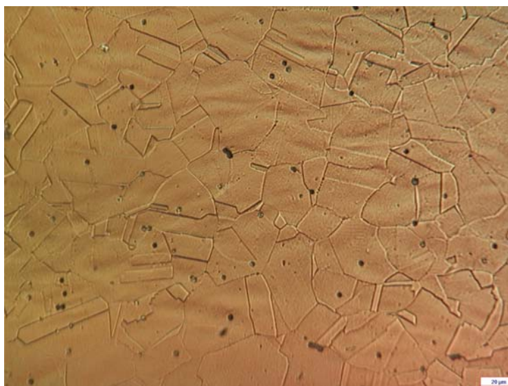
Figure 1. The austenitic microstructure of HAS 1 grade. Etching: 1:1/HCl:HNO 3
