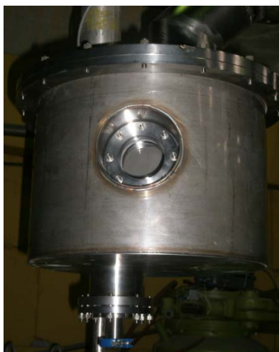
Fig. 6. Chamber-imitator of the test stand with glass window and vacuum jacket.
