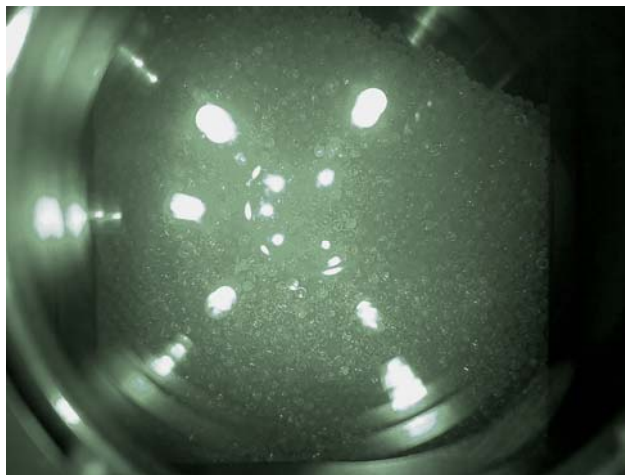
Fig. 8. Photo of delivered beads in the chamber (18 cm x 18 cm x 4 cm) taken by the video camera (The temperature of beads is about 50 K, amount is about 27000).
