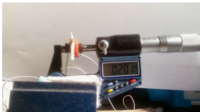
Fig. 1. The electrochemical cell used for the determination of ionic conductivity of acrylic ion exchange membranes.
