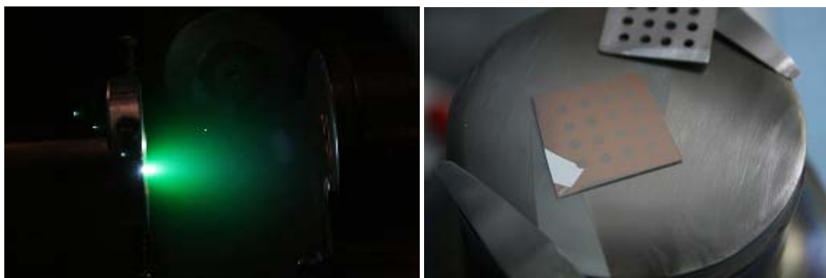
Fig. 3. Deposition of thin layers of Co / Cu on Sital sub-layer using mask.
