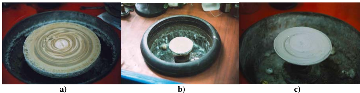
Fig. 1. Different types of polishing machines pads a) Pad of polishing machine with SiC powder; b) Pad of polishing machine with diamante powder; b) Pad of polishing machine with \text{Al}_2\text{O}_3 powder.
