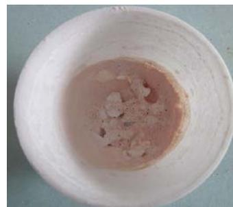
**Fig. 2. Synthesized CaZnO<sub>2</sub>-I at 600 °C.**
