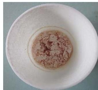
Fig. 3. Synthesized  $\text{CaZnO}_2$ -II at  $600\text{ }^\circ\text{C}$ .
