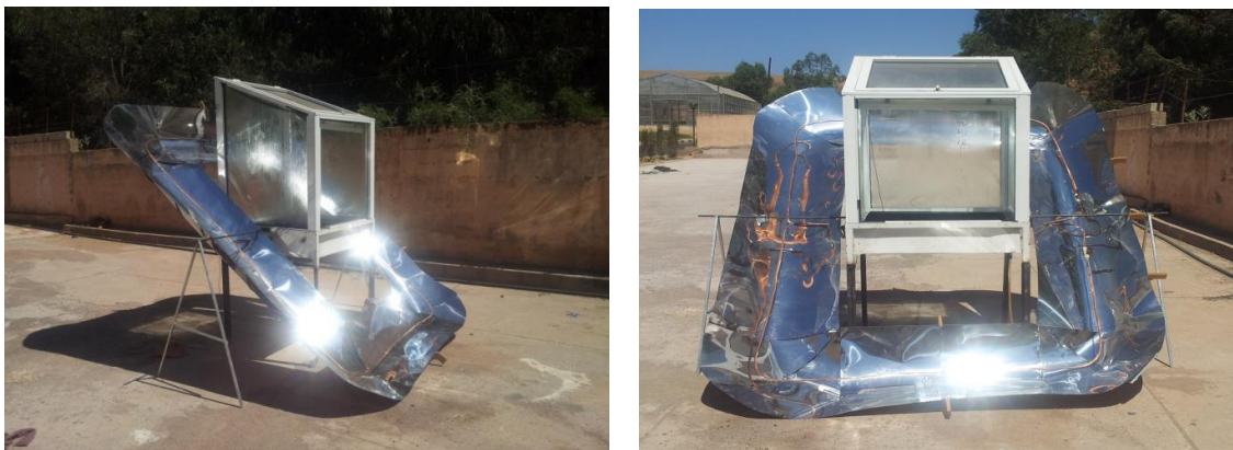
Figure 8. Greenhouse Solar Distiller Coupled With Parabolic Trough.
