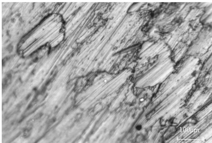
Figure 8. Visualization of discontinuous transformation of crude casting alloy Pb 2% Cd 1% Bi 2% Mg tempered with water at 20°C during overaging after 3 days of quenching.
