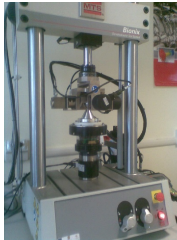
Figure 3. MTS Bionix axial testing system equipped with a hip test fixture.
