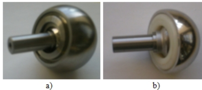
Figure 4. Implants tested on the MTS Bionix load unit: a) prototype, b) conventional implant.
