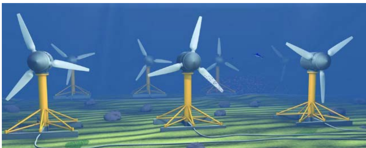
Figure 2. Horizontal Axis Marine Current Turbines
