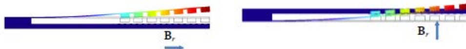
a) The magnetic forces raise the PI blade b) The magnetic forces press the PI blade.
