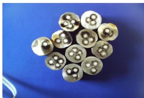
Figure 1b). The steel samples spectrochemically investigated.
