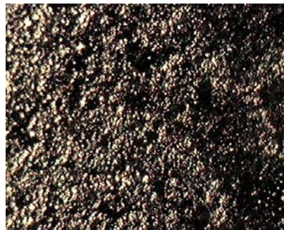
Figure 6. Morphological aspects of a sparking surface; marginal area of a sparking surface.
