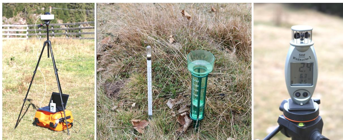
Figure 2. Instrumentation used for measurements of solar radiation fluxes, relative humidity, temperature, rainfall and wind parameters during floristic surveys performed in Fundata, Romania – year 2017.
