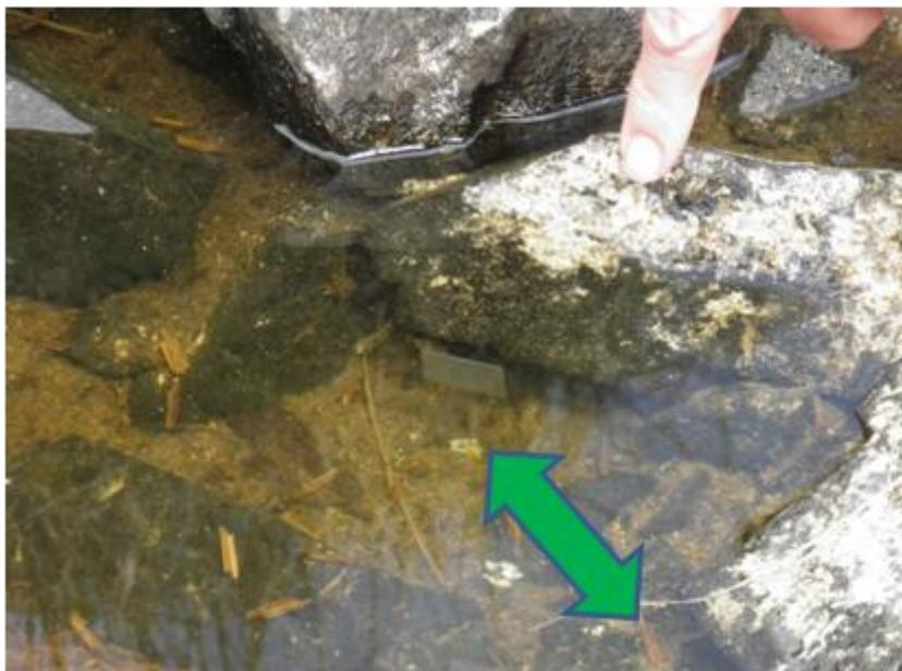
Figure 1c. Actual setup (Mongolia, June 2017). Small depression (diameter about 1.25 m, 90 cm deep, little light getting in) in a drying bog, N Mongolia. Marks point to chitin-plates on glass support, exposed to water (left) and sediment (bottom right). Photograph by Beate Noack.
