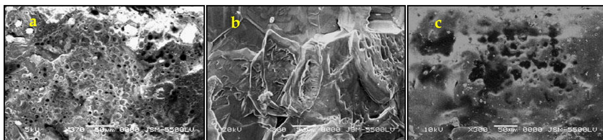
Figure 7. SEM of granite samples treated with Paraloid B 44: a) initial; b) after thermal ageing; c) salt ageing.
