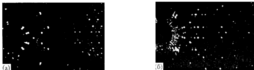
Figure 1. X-ray patterns of the oscillation around the axes a (a) and b (b) of \text{Tl}(\text{InS}_2) single crystals 0.985(\text{FeSe}_2)0.015
