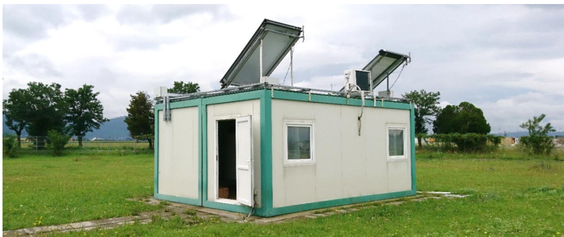
Figure 1. The outdoor testing rig for solar thermal collectors considered in the study.
