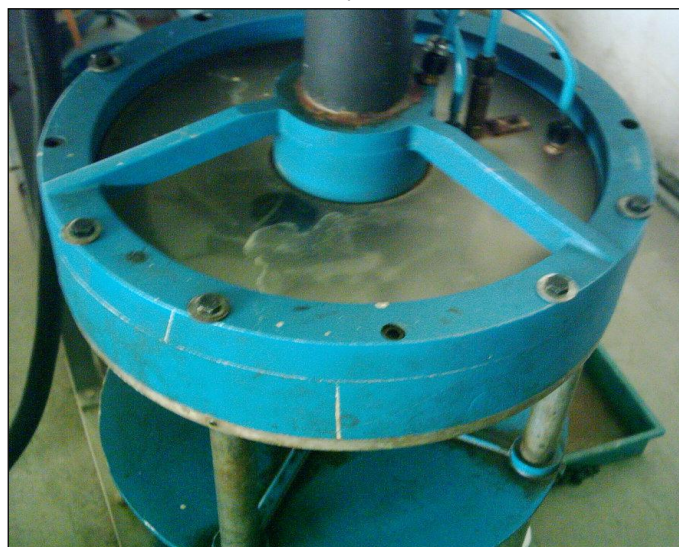
Figure 8. Appearance of cavitation phenomenon in the centrifugal test pump.
