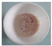
Fig. 2. Synthesized CaZnO<sub>2</sub>-I at 600 °C.
