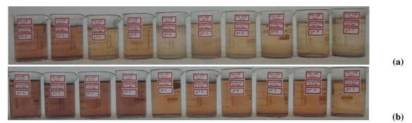
Photo 3. Effect of pH on the photocatalytic degradation of textile effluent at 120 minutes [textile effluent = 3%, (a)= CaZnO<sub>2</sub>-I, (b)=CaZnO<sub>2</sub>-II].
