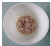
Fig. 3. Synthesized CaZnO<sub>2</sub>-II at 600 °C.
