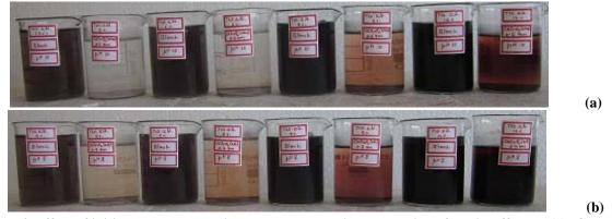
Photo 4. Effect of initial dye concentration on photocatalytic degradation of textile effluent [(a)= $CaZnO_2$ -I/pH= 0.6g/10, (b)= $CaZnO_2$ -II/pH= 0.7g/8].
