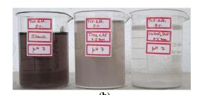
Photo 1. Rate of degradation of textile effluent at 120 minutes [(a)=Tex.eff./TiO<sub>2</sub>/CaZnO<sub>2</sub>-I, (b)=Tex.eff./TiO<sub>2</sub>/CaZnO<sub>2</sub>-II].
