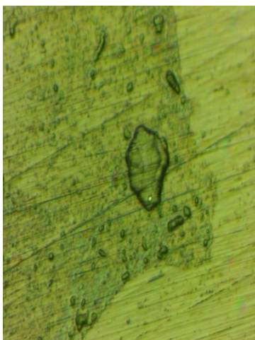
Figure 19. Visualization of the structure of the G30 alloy treated at 700°C, attacked with aqua regia, after 68 days from quenching.
