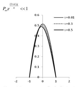
Figure 6. Temperature profile for fixed values of  $\alpha$ =1,  $\Gamma_d$ =0.2, Gr= 0.4, and for various values of v
