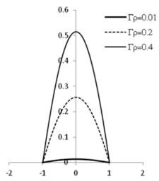
Figure 7. Temperature profile for fixed values of  $\alpha=1$ ,  $\Gamma_r=0.2$ ,  $\nu=0.01$  and for various values of  $\Gamma_r$
