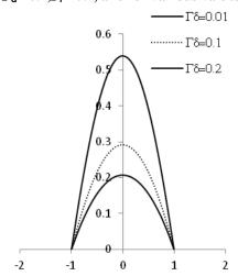
Figure 4. Temperature profile for fixed values of  $\alpha$ =1,  $\Gamma_{\rho}$ =0.2, v= 0.01 and for various values of  $\Gamma d$
