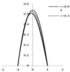
Figure 2. Temperature profile for fixed values of  $\alpha=1$ ,  $\Gamma_d=0.2$ ,  $\Gamma_r=0.4$ , and for various values of v
