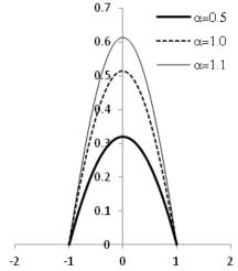
Figure 5. Temperature profile for fixed values of  $\Gamma_r$ = 0.04,  $\Gamma_d$ =0.2, v= 0.01 and for various values of  $\alpha$
