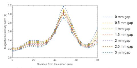
Figure 8. Radial variations of magnetic flux density generated by a concentric permanent magnetic ring.
