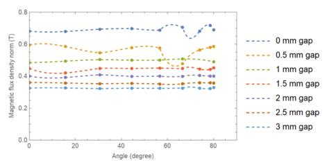
Figure 9. Angular variations of magnetic flux density generated by a concentric permanent magnetic ring.
