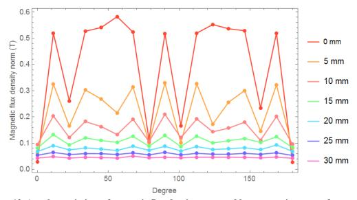
Figure 12. Angular variations of magnetic flux density generated by concentric arrays of permanent magnets at varying distances in the Z-axis up to 30 mm.
