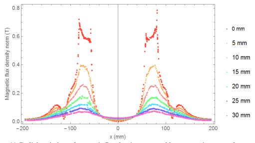
Figure 11. Radial variations of magnetic flux density generated by concentric arrays of permanent magnets at varying distances in the Z-axis up to 30 mm.
