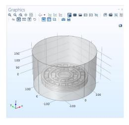
Figure 3. Geometry of array of magnets arranged into concentric rings.
