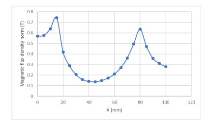
Figure 5. Radial variations of magnetic flux density generated by a permanent magnetic ring.
