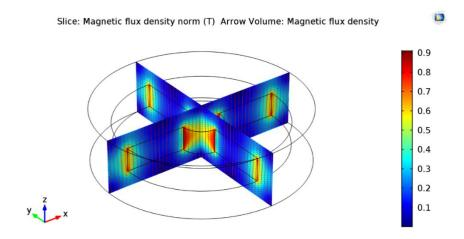
Figure 4. Profiles of magnetic flux density generated by a permanent magnetic ring.
