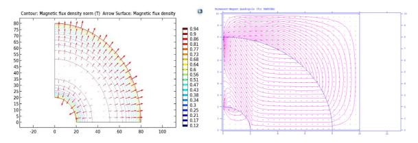
Figure 6. Magnetic flux contours simulated COMSOL Multiphysics 5.3 and Poisson SUPERFISH 7.0.
