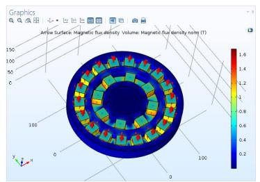
Figure 10. Profiles of magnetic flux density generated by concentric arrays of permanent magnets.
