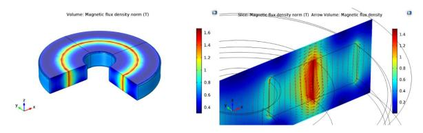
Figure 7. Profiles of magnetic flux density generated by concentric permanent magnetic ring.
