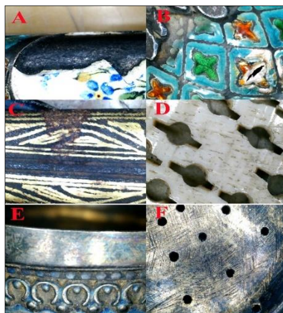
Figure 5. Portable digital microscope photomicrograph of the metal with (500X magnification) shows: (A, F) Black tarnish, (B) Cuts in the metal, (C) Corrosion in some parts, (D, F) scratches in ivory and metal.
