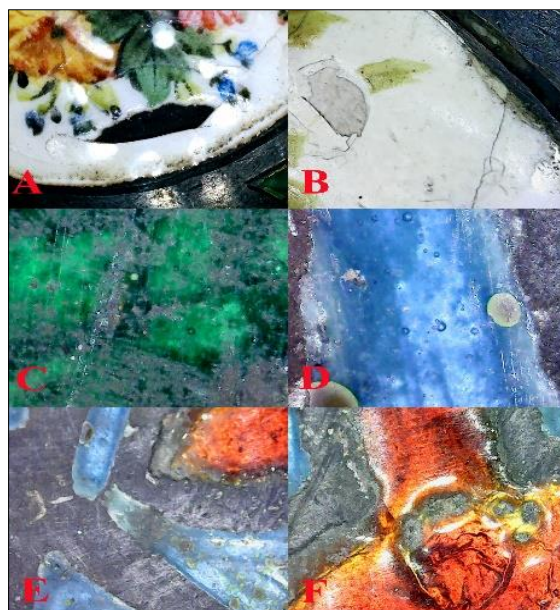
Figure 4. Portable Digital microscope photomicrograph of the enamel with (500X magnification) shows: A. loss of enamel, B. cracks and loss of Limoges enamel, C. scratches, D. pits, E. color change, F. loss of champlévé enamel.
