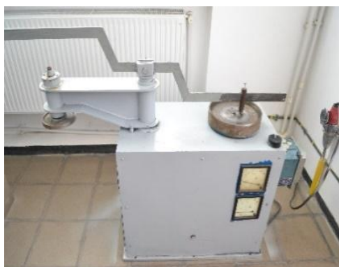
Figure 11. Installation for determining the wear rate.
