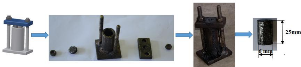
Figure 4. The mold for obtaining samples for assessing tribological behavior.
